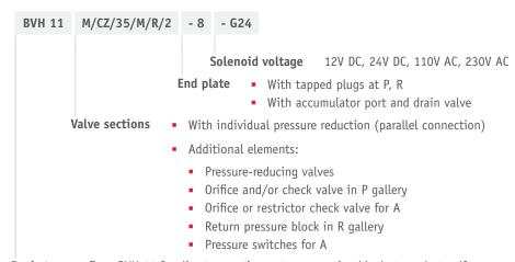
**Basic type** Type BVH 11 for direct mounting onto connection blocks type A etc. (for compact hydraulic power packs type KA, MPN, HC, HK, HKF, HKL)
